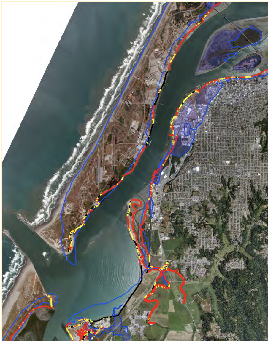
Figure 3. Eureka Bay, shoreline areas overtopped by 3 feet of SLR (red), 6 feet (yellow) and the 1870 tidal inundation footprint (blue). See the Humboldt Bay Shoreline Inventory, Mapping and Sea Level Rise Vulnerability Assessment Report.
