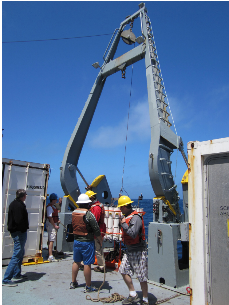
Researchers deploy a conductivity-temperature-depth (CTD) rosette. Photo: Sara Shen.
