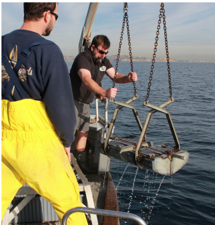
A Bight '13 field crew collects seafloor sediment using a grab sampler. Photo: SCCWRP.
