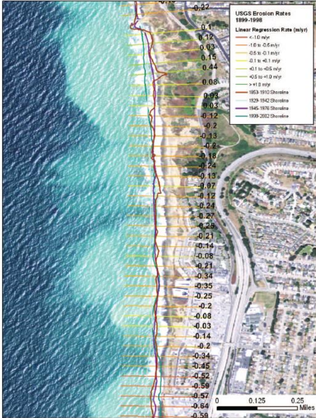
Figure 3.10 Historical Coastal Erosion Rates Derived from USGS using DSAS. The Location is the same as shown in Figure 3.9
